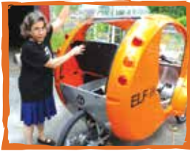
The ELF bike can travel 20mph on electric power only and up to 30mph when combined with pedaling.
