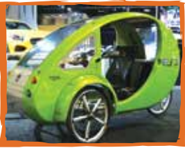
The ELF bike can travel 20mph on electric power only and up to 30mph when combined with pedaling.
